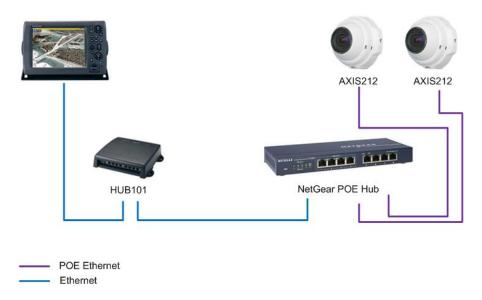
IMPORTANT: Never connect a POE port to the HUB101. Always use one of the NON-Powered ports to connect the HUB101 to the POE Hub.
