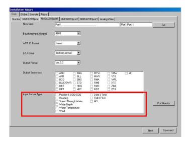
Example: If you connect a sensor such as a PB100 which provides Wind information but also Position, you will have to check "Position & SOG/COG" as well as "Wind". You can click on the "Port Monitor" Button to make sure that the sensor is correctly sending the corresponding Data.
