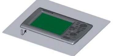
2. Pull the tool to raise the panel slightly. Repeat this action for all notches on the lower side of the unit
