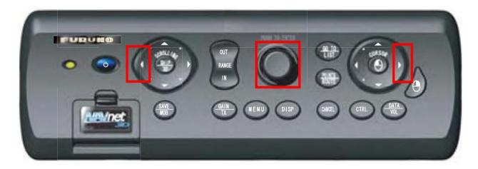
The Keyboard will beep two times. You can release the button at this time. The keyboard will now control the MFDBB.
