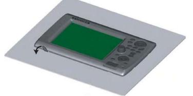
3. Insert the tool into the small notches located on the sides of the panel, and pull the tool to raise the panel slightly
