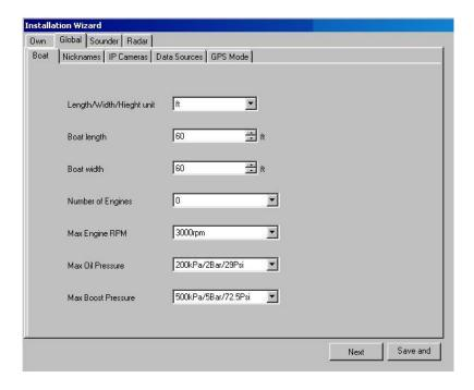
When an Engine(s) with a NMEA2000 Port is connected to an MFD in the network, the Maximum Value of the RPM, Oil and Boost pressure needs to be set up in order to correctly adjust the scale of the Analog Engine Gauges.
