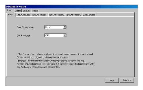
Please refer to the "External Monitors" paragraph on p.37 for more information on Clone and Extended mode when two monitors are connected to a single MFDBB processor.
