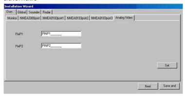
Note: The Analog Video inputs are only available on the MFD where they are connecting to. Unlike the IP Camera, these video feeds are not available on the network
