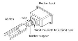
7. Slide the rubber stopper into the hole of the rubber boot, and fasten the cable tie to hold the rubber boot and stopper.
