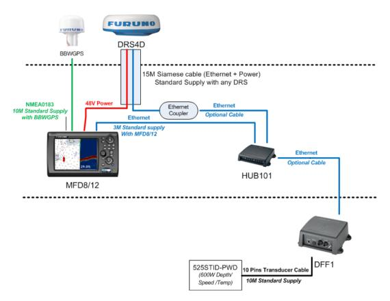
Additional Furuno Network Sensors can also be plugged directly to the HUB (using a regular Ethernet cable):
