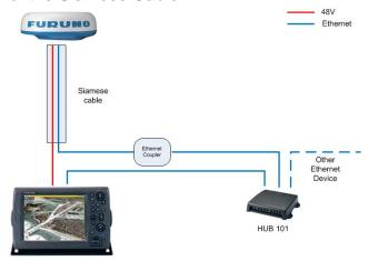
Example of straight Ethernet Coupler (FUSA P/N= RJ4-5CN-STR):
