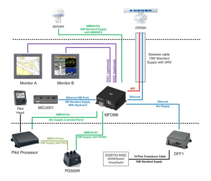
In the above example, the MFDBB is configured for Extended Mode. The two monitors show independent screen displays that can be configured independently. Only one Keyboard is used to control both monitors (the cursor will "jump" back and forth from monitor to monitor). The two screens need to be located in close proximity to each other.
