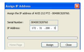
You will need to restart (power OFF and ON) the camera after the address is changed. (Just unplug and plug back the Ethernet cable if you are using the POE).
