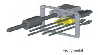
3. Attach each connector to the appropriate location at the rear of the display unit.
