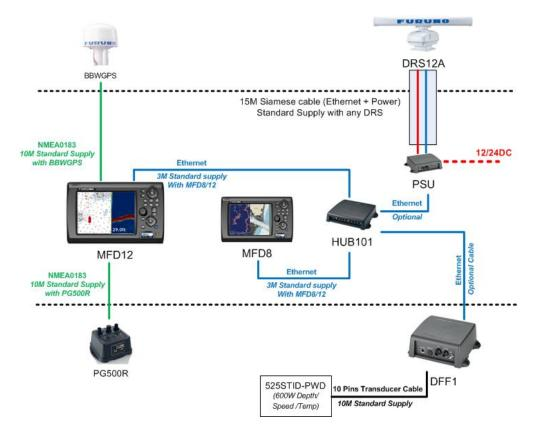
Additional sensors can also be plugged directly to the HUB (using regular Ethernet cable):
